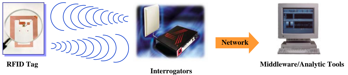
Figure 5.3: Key elements of an RFID system
