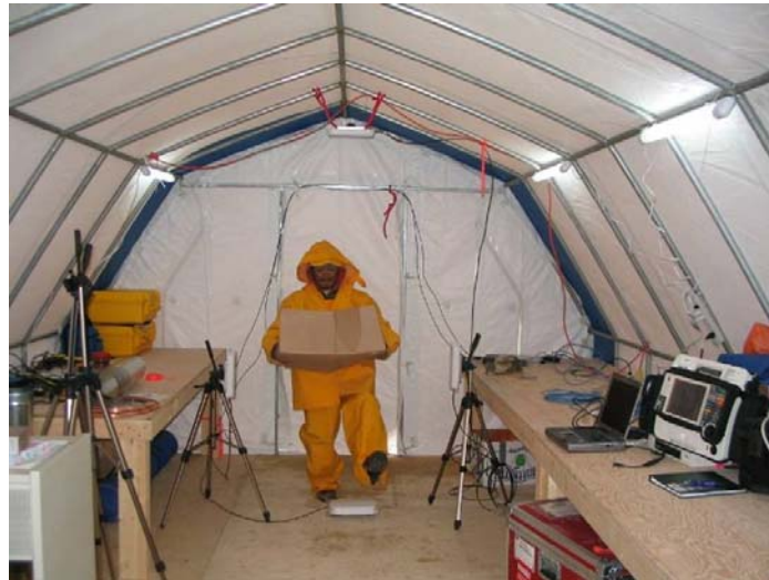
Figure 5.5: One of our volunteers, Samson Simeon, carrying out one run of the formal RFID experiment. Four antennas are mounted (left, right, top, bottom) forming a gate.
